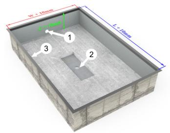
side of the lift table. 2- Drainage holes where required. This is centre of the pit
